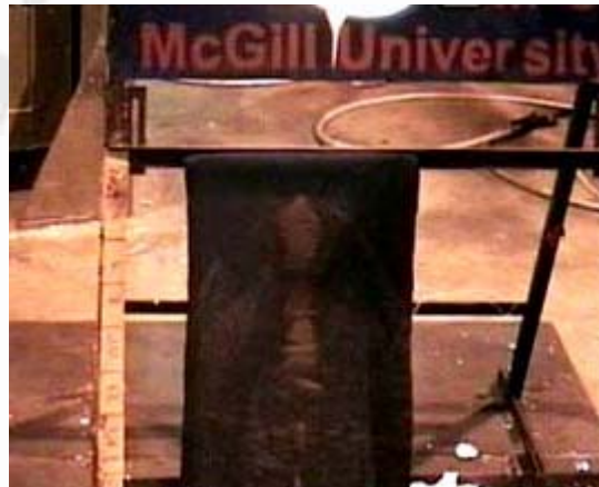
Appearance of the fabric without any breakage or combustion. No metal mass adhered
